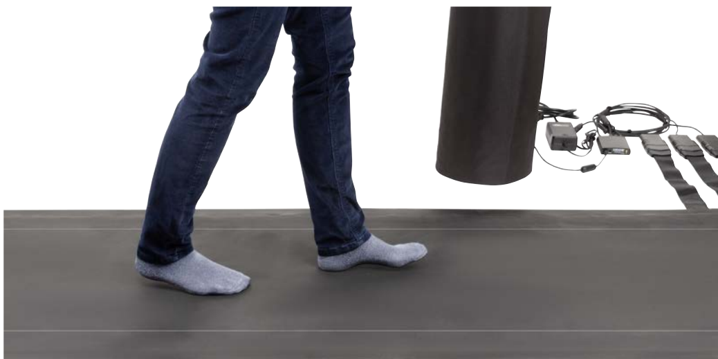
Figure 10. The XSENSOR Walkway mat
